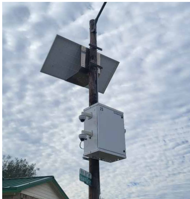
Pictured above: Solar powered construction site security camera system mounted to a forklift carry steel skid. | Solar powered safety lighting on forklift-ready steel skid. Pictured below: Solar powered camera system mounted to existing light pole.
